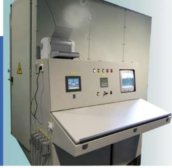
A purpose-built load bank for the performance testing of engines and generators of all types of diesel electric locomotive up to 4000hp
