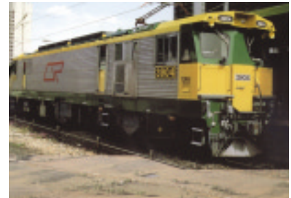
Class 3900 Locomotives, Queensland, Australia: 80 braking resistors @ 2MW
