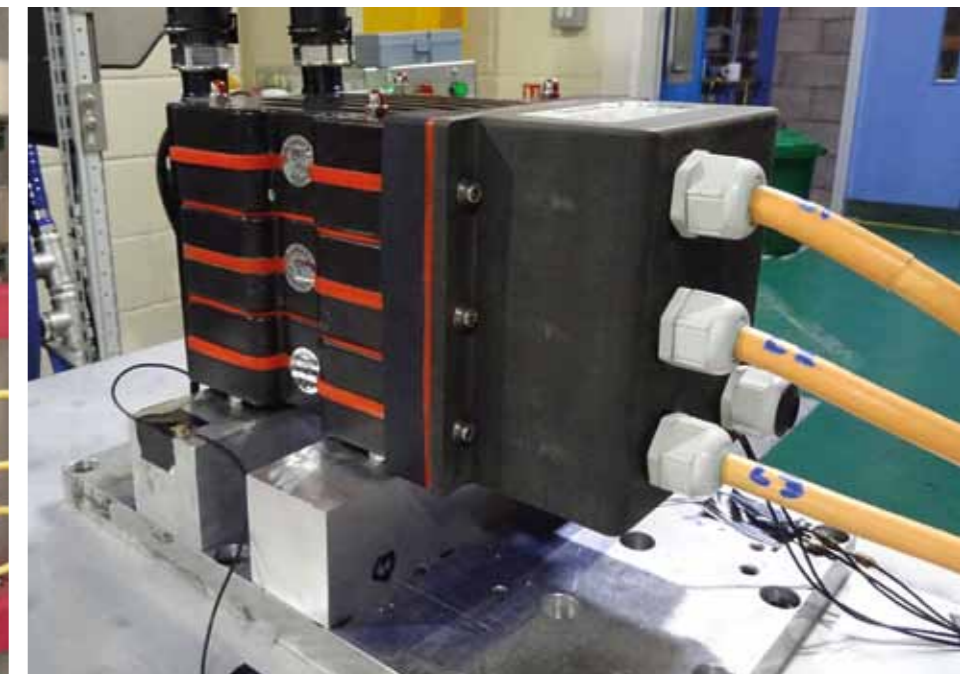
Shock and vibration testing with simultaneous power cycling being carried out to current automotive and traction standards.
