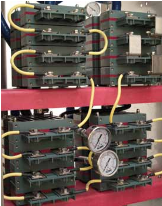
Multiple EV2 units assembled to provide a single 400kW water cooled load
