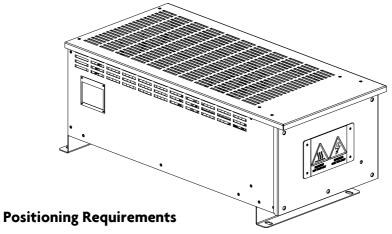
The enclosure must be mounted on a flat surface, ideally horizontally.
